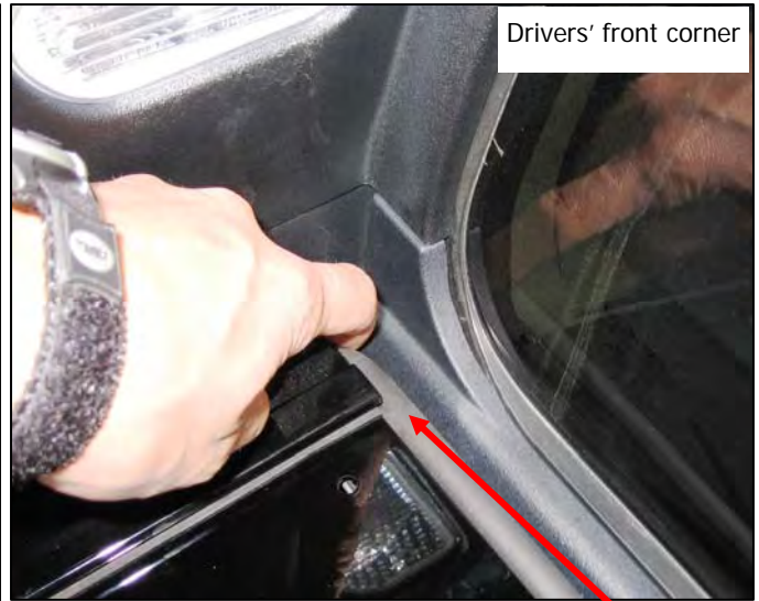
Fig. 11b Position front covers weather-strip.
